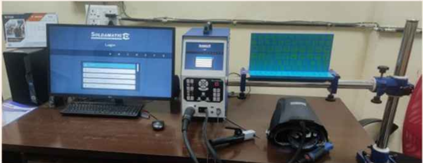
WELDING SIMULATOR SETUP
